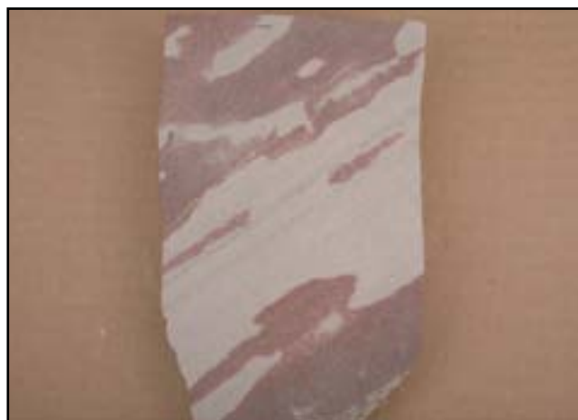
Mereenie Sandstone at 1211 m in Dalmatia 1. Width of core is 95 mm. Photo 042438.
