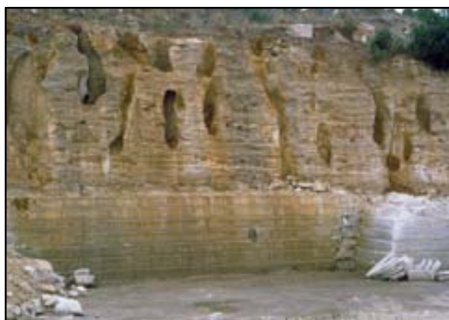
Gambier Limestone with solution pipes at Steetley building stone quarry near Mount Gambier. Photo 042492.
