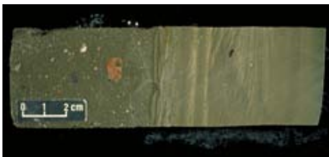
Finely developed foreset beds in silty sandstone with minor pebbles, overlying diamictite containing clasts of igneous rocks, Coolardie Formation at 243.14–243.28 m in Lock 1. Top is to the right. Photo 042446.
