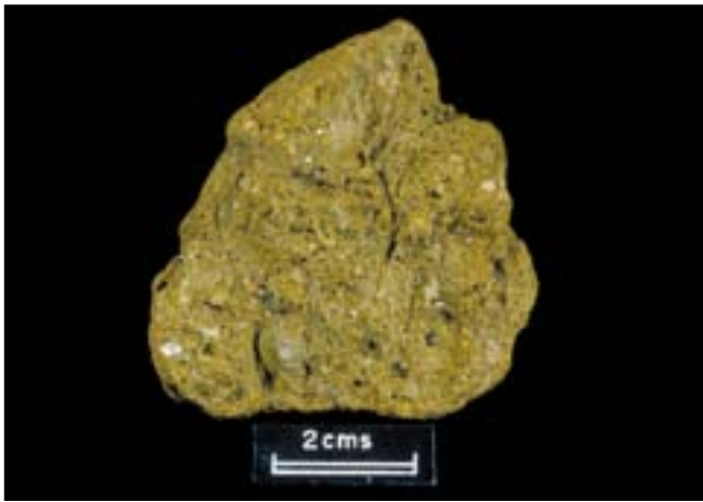
Sample of kimberlite from Calcutteroo, near Terowie. Phlogopite laths 0.5–3 mm across are set in a groundmass of fine-grained phlogopite, clay and serpentine. An ovoid autolithic xenolith is at the base of the specimen. Photo 024578.
